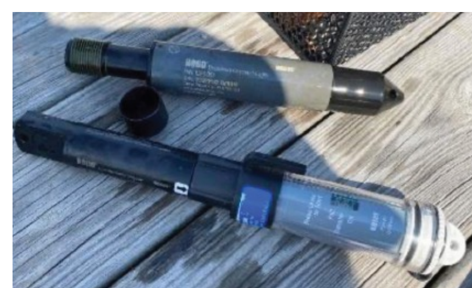
Figure 2. New accurate and low-cost environmental sensors like these dissolved oxygen and salinity loggers made by our project partner Onset Computer create new opportunities for continuous water quality data collection. They also create new challenges for organizations to maintain sensors and manage much larger amounts of data.
