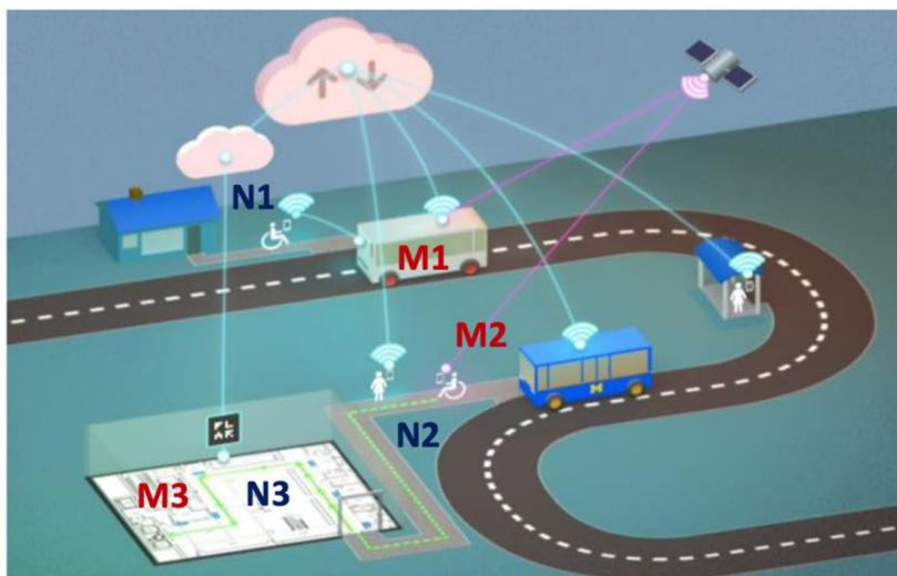
NAVIGATION TASKS: N1: House to transportation pickup point N2: Drop off point to entry of building N3: Entry of building to desired room
