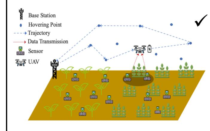
DRONE optimally selects a subset of sensors to visit within the UAV's energy capacity and estimates the observed measurements generated by other sensors.
