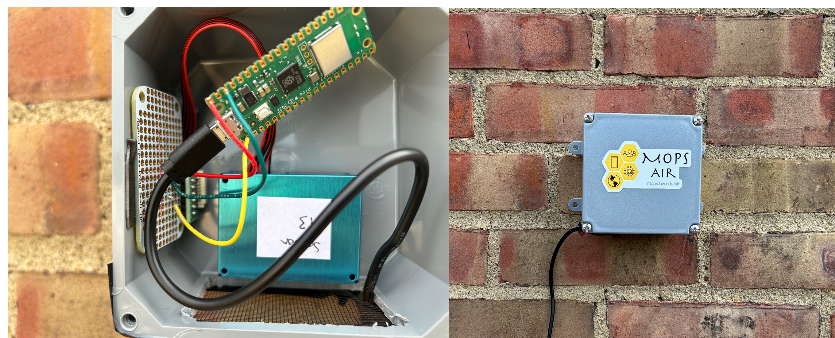
Figure 3 – Test sensor deployed on our campus using both MicroPython and CircuitPython in an electrical enclosure.
