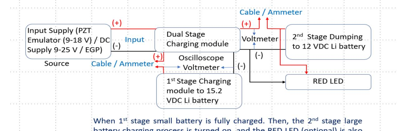
battery charging process is turned on, and the RED LED (optional) is also turned on. Otherwise, the RED LED and 2nd stage battery chaging process always stay turned off.
