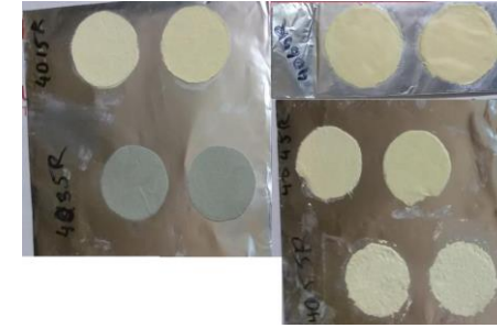
PZT Composite Cell Growth on Al
